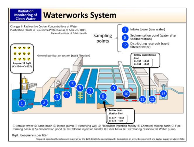
This figure shows the rapid filtration method, which is generally used in Japan. In this method, chemicals are injected into raw water taken from a river or dam to cause sedimentation of mud and small particles and make them into big chunks called "floc." Tap water is created by filtering the clear upper portion of such water.
