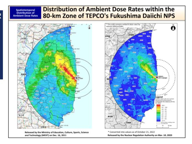
In order to ascertain the changes in the effect of radioactive materials, the airborne monitoring survey has been conducted continuously within the 80-km zone of Tokyo Electric Power Company (TEPCO)'s Fukushima Daiichi NPS, and the distribution of ambient dose rates and deposition of radioactive cesium have been surveyed. Additionally, the effect of radioactive materials outside the 80-km zone has also been ascertained through the airborne monitoring survey.
