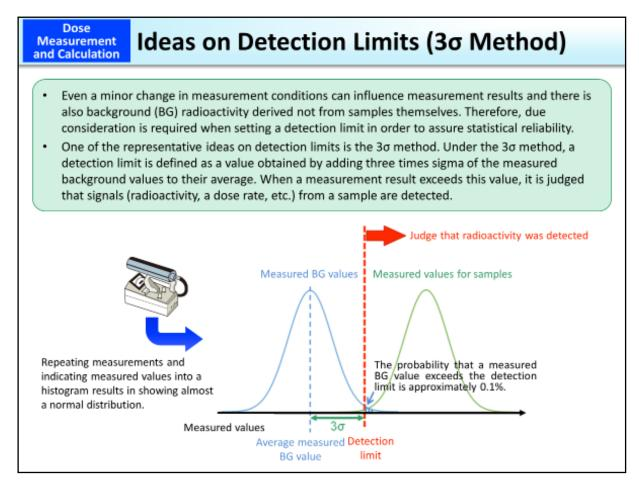
When measuring background radioactivity or dose rates using a survey meter or other equipment, even a minor change in measurement conditions can influence measurement results. Therefore, it is necessary to repeat measurements in order to obtain reliable measurement results.
