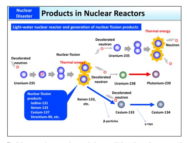
The light-water nuclear reactor is currently the most widely used type of reactor around the world (also used at Tokyo Electric Power Company (TEPCO)'s Fukushima Daiichi NPS). Bombarding enriched uranium fuel (Uranium-235: 3-5%; Uranium-238: 95-97%) with neutrons results in nuclear fission. Radioactive nuclear fission products such as lodine-131, Cesium-137, and Strontium-90 are created in this process. When Uranium-238 is bombarded with neutrons, Plutonium-239 is created.
