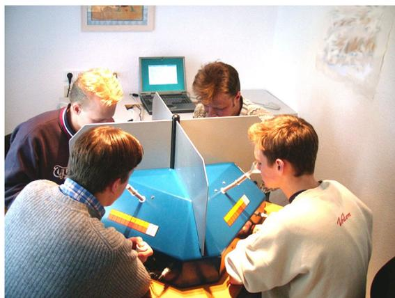
Fig. 4 Example of a four-sniffing-place yes/no olfactometer (in total 4 sniffing ports)
