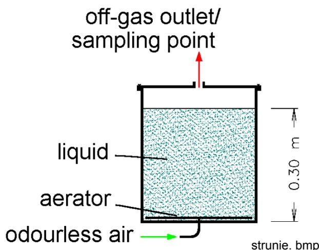
Fig. 5 sketch of the OEC test reactor
