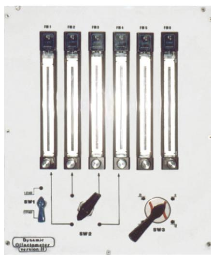
Figure 2. An upgraded version II dynamic olfactometer
