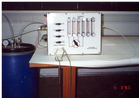
Figure 1. Manual dynamic olfactometer
