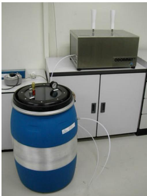
Figure 3. Computerised dynamic olfactometer (Odormat)
