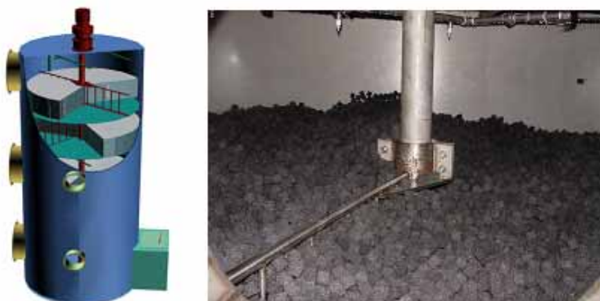
Figure 4. Mechanical stirring device to prevent a clogging in a biofilter
