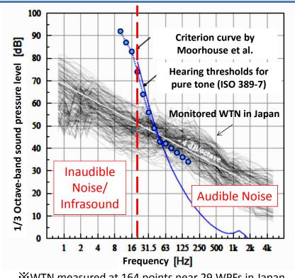
WTN below 20 Hz did not exceed the hearing thresholds of ISO 389-7 or Criterion curve
