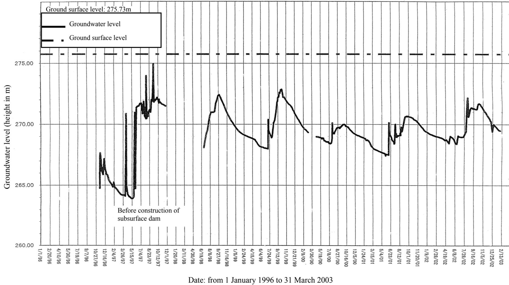
Fig. 6.4: Results of continuous observation of reserved groundwater level by the subsurface dam (at observation well P-4)
