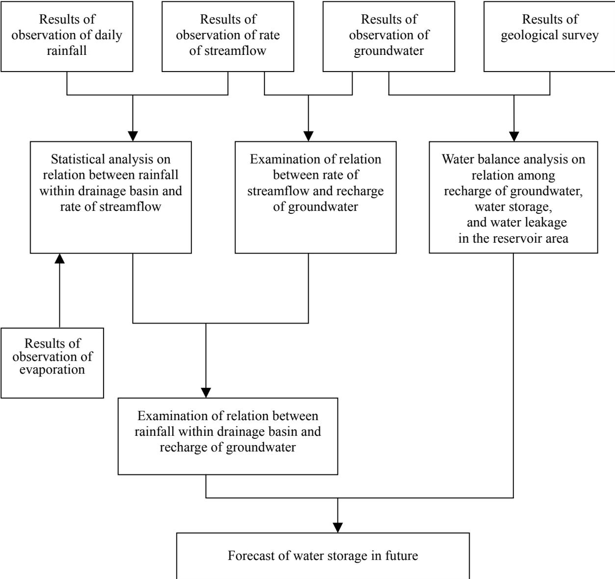
Fig.6.7: Flowchart of analysis of the water-storage mechanism
