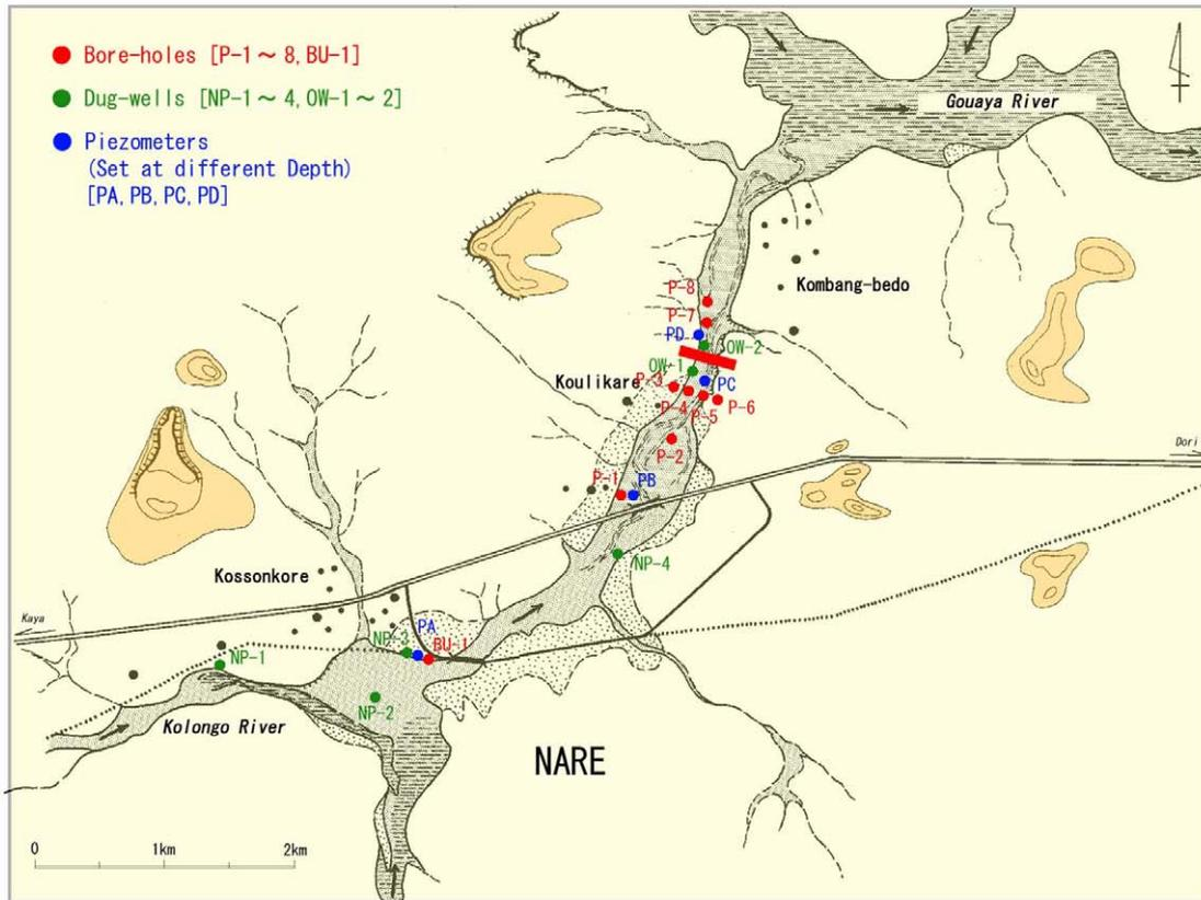
Fig. 6.1: Schematic diagram of the distribution of facilities for groundwater observation
