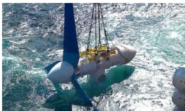
図 6-1-3(c) A turbine for the MeyGen tidal stream project
