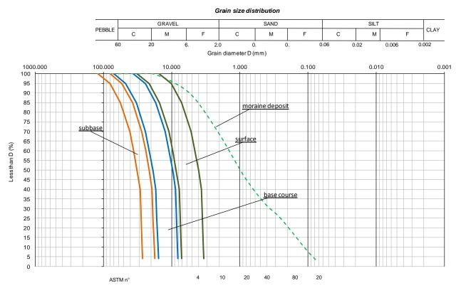
Figure 2.16: Sub-base, base course, surface Grain size distribution and relative layers
