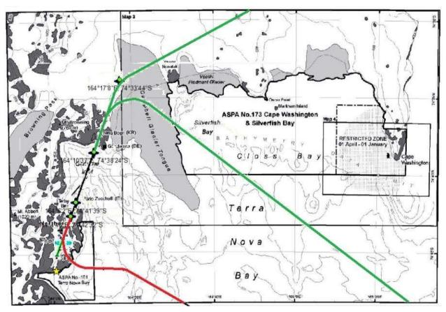
Figure 5.2: The area around MZS with the planned flight routes. Operative landing/taking off and of emergency missed approach (green and red lines respectively), over layered with bird colonies (yellow star) and ASPA 161/173 borders (black lines).
