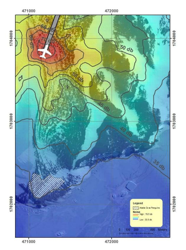
Figure 5.1: Estimated noise level over natural noise condition (20 dB(A)) at 125 Hz, during full engine power of Hercules L100/30, in take-off procedure.
