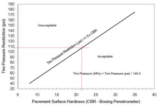
Figure 2.21: Tire Pressure Restriction vs CBR Measured with Boeing Penetrometer [2.7].
