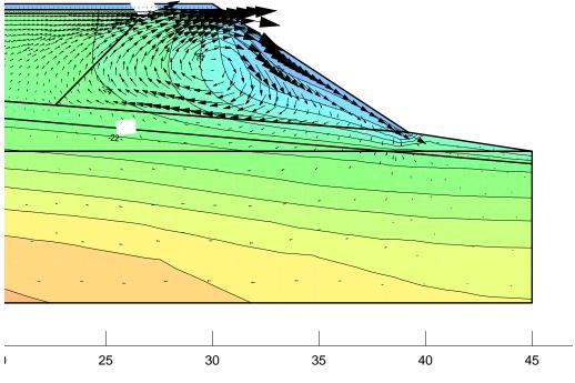
Figure 2.26: Numerical result – convective cells and temperatures (Day 220).
