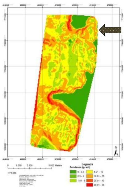
Figure 3.5: A slope map of the area around the station and the alternative location for the airstrip at Campo Antenne (black arrow).
