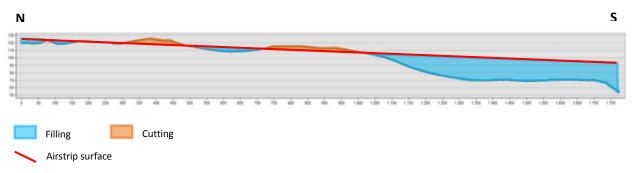
Figure 3.8: A slope cut of a possible airstrip 1770 m long at Campo Antenne
