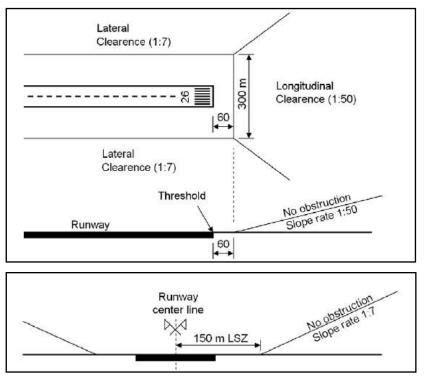
Figure 3.9: Behaviours of flight clearance surfaces at Campo Antenne
