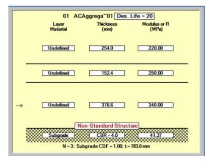
Figure 2.19: FAARFIELD software results for a subgrade with a reduced CBR=6% [2.6].
