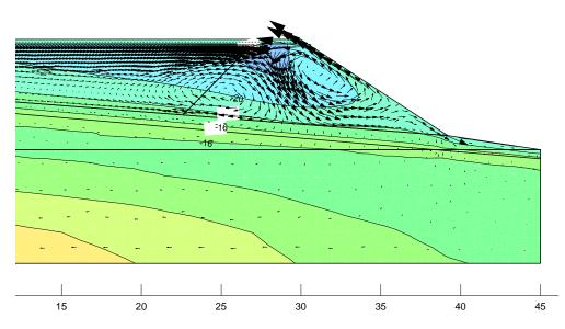
Figure 2.27: Numerical result – convective cells and temperatures (Day 270).
