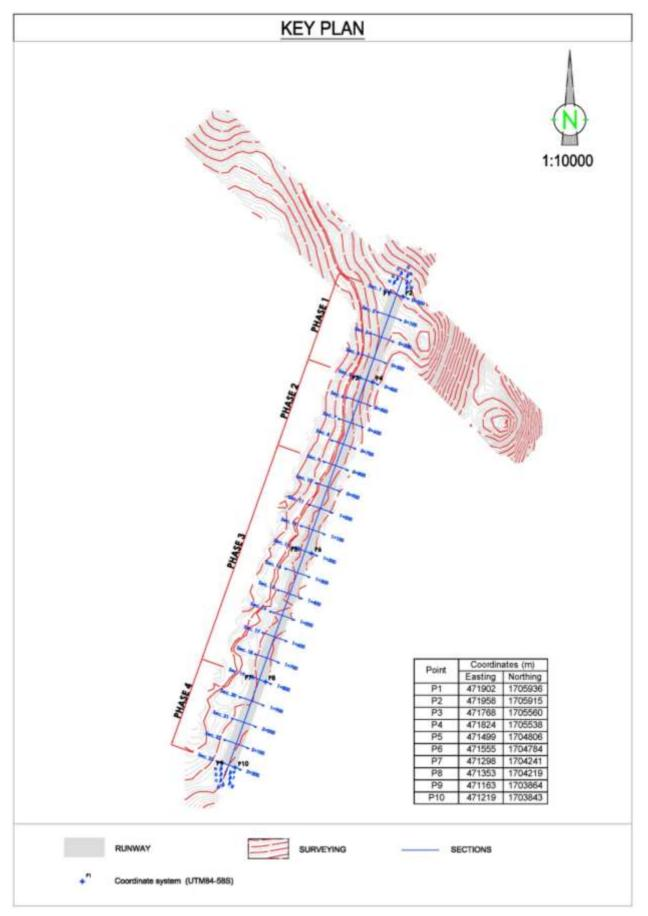
Figure 2.5: Runway layout with the four construction phases.
