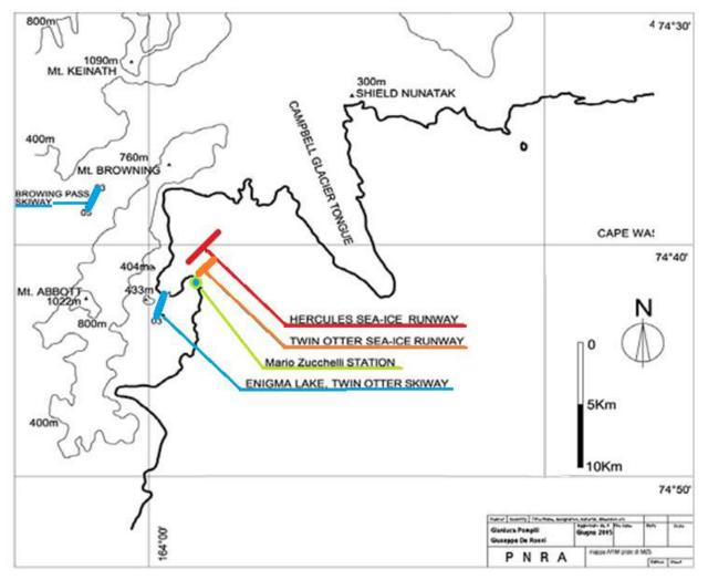
Figure 3.1: Locations of the available icestrips around MZS (red line for the Hercules icestrip and blue/orange lines for Twin Otter icestrip/skiways respectively)
