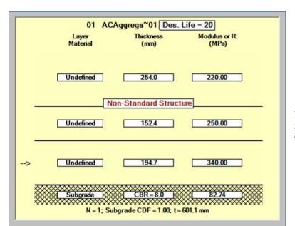
Figure 2.18: FAARFIELD software results for a subgrade with a reduced CBR=8% [2.6].
