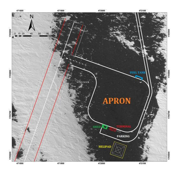
Figure 2.6: Runway facilities: Apron, taxiways, fuel tank, helipad, and vehicle access road.
