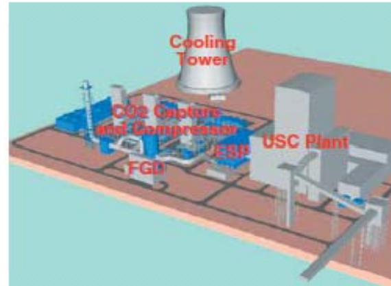
Result of FS on 500 MW USC + CCS
