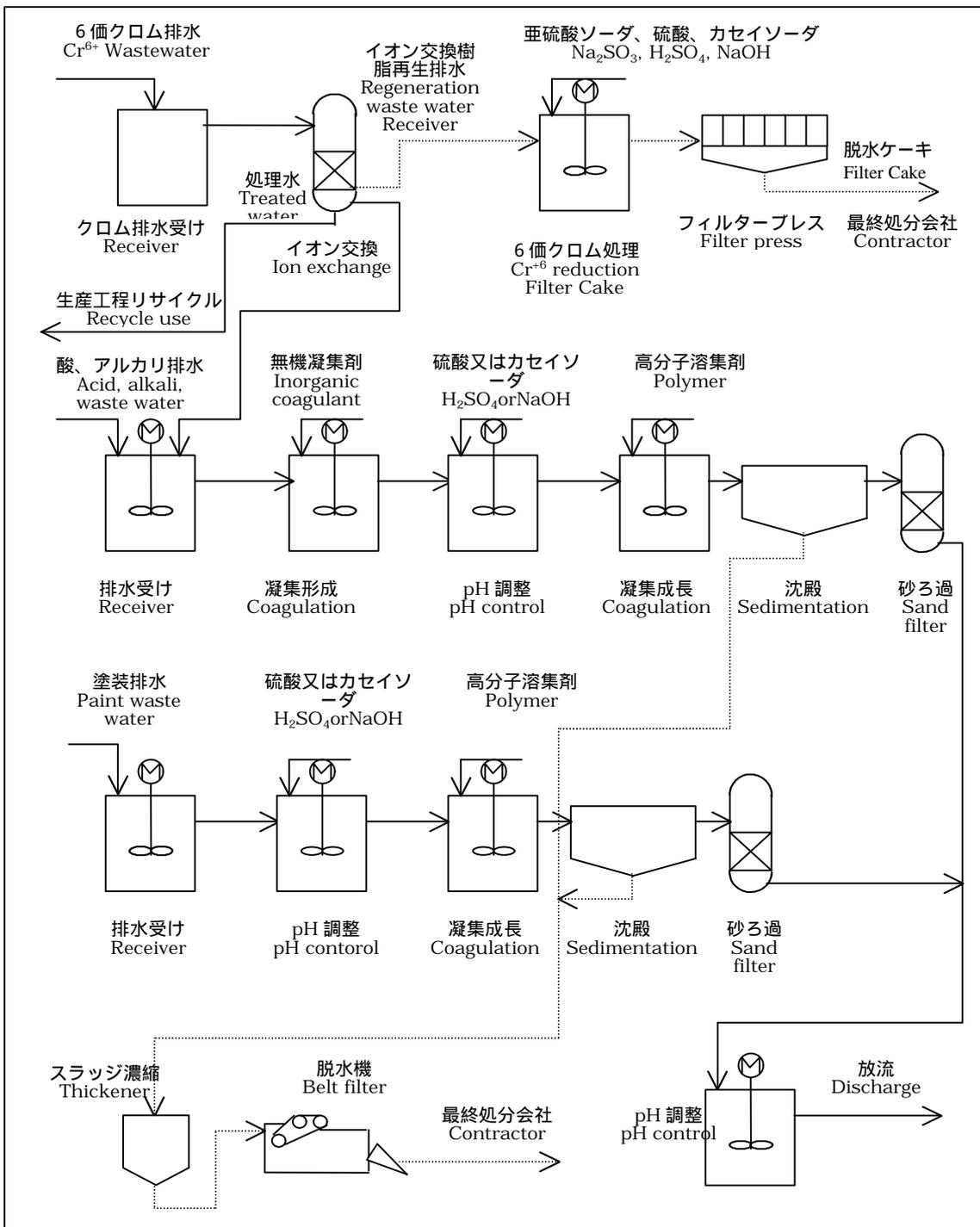
The pH value of the wastewater from the painting process is adjusted at first. A coagulant is added to the wastewater to coagulate and settle the suspended solid. The fine suspended particles that still remain
