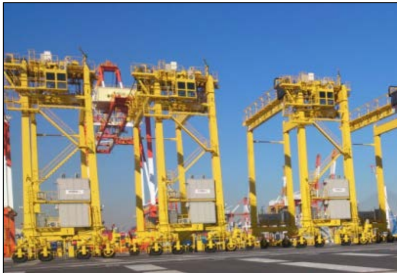
Figure 35 Hybrid RTGs Used at Yokohama Port Beige-colored box-shaped objects near bottom are batteries.
