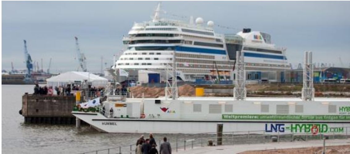
Figure 56 Barge Generating Power with LNG for Supply to Ships (Front) (Hamburg)
