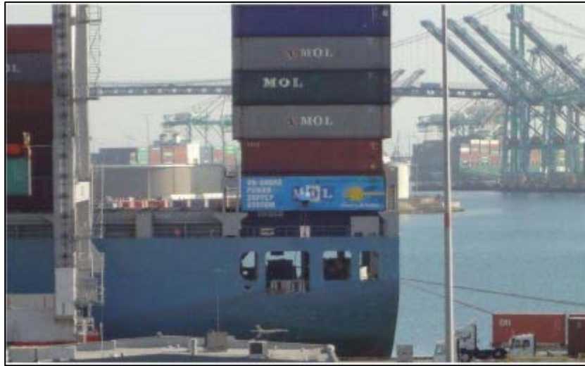
Figure 54 Ship Receiving Power Loaded with Containers for Shore Connection System (Los Angeles)
