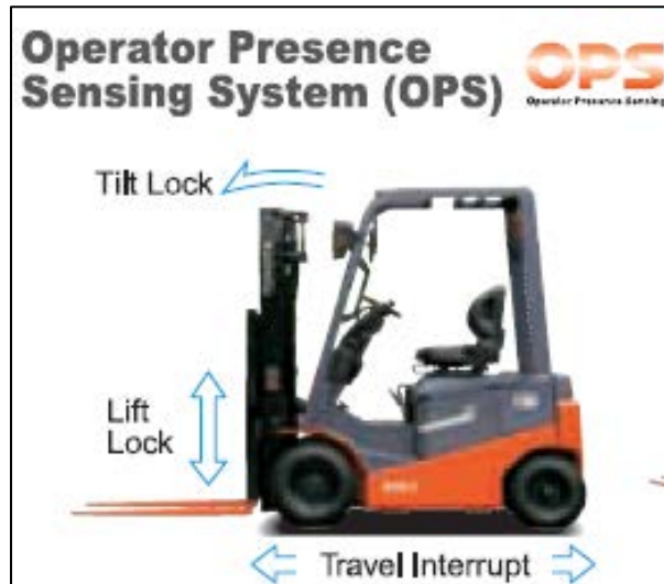
Figure 28 Mechanism of Operator Presence Sensing System
