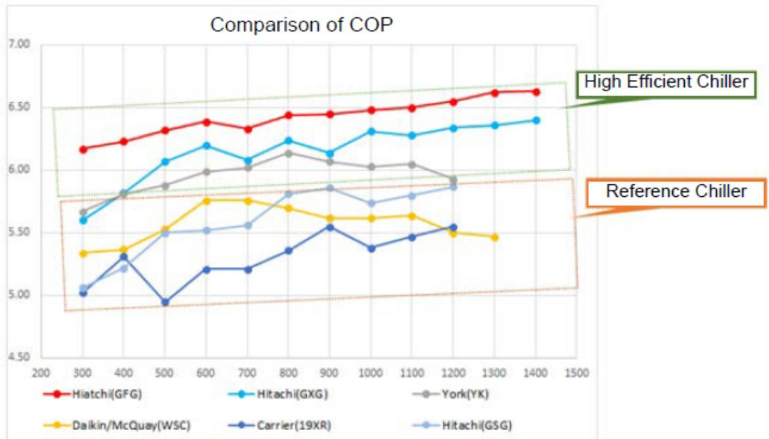
Figure 3.3.2-5 COP comparison of Hitachi GFG and reference equipment
