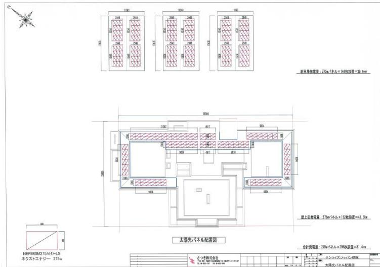
Figure 3.2.2-11 Assignment of solar panels (Sunrise Japan Hospital)
