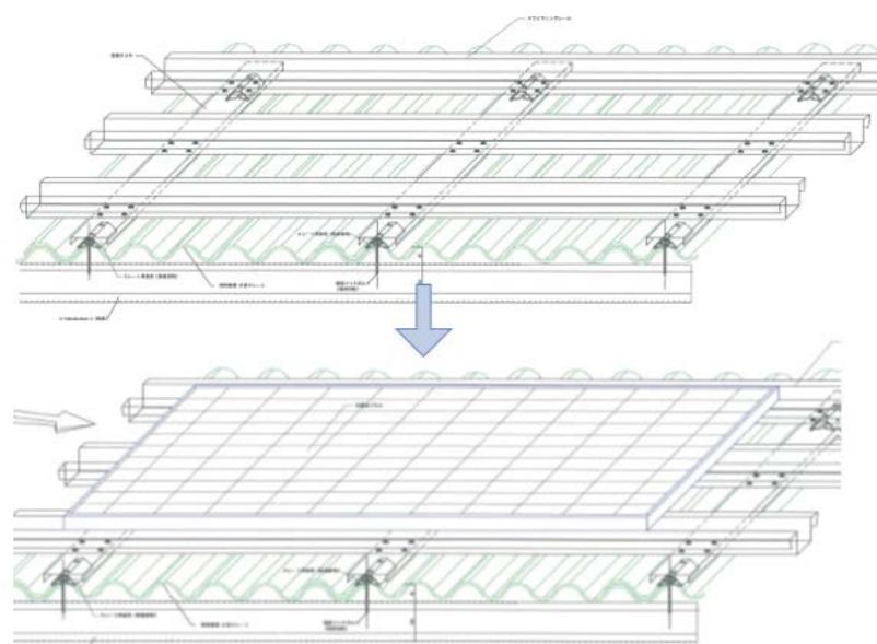
Figure 3.2.2-10 Ultra light installation method (slate roof)
