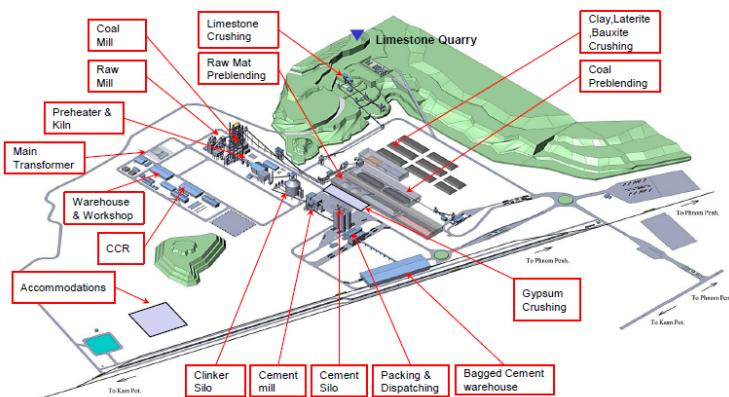
Figure 3.4.2-1 General layout of cement factory
