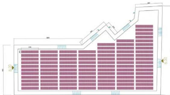
Figure 3.4.2-9 Examination A) Install solar panels across the water pond
