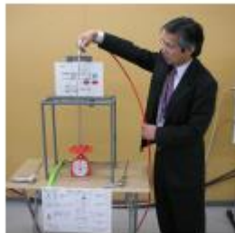
Comparison of pressure loss between direct cutting edge of pipe and blow gun
