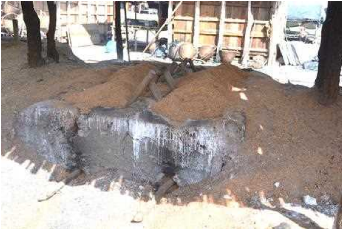
Photograph Salt making furnace with sawdust added
