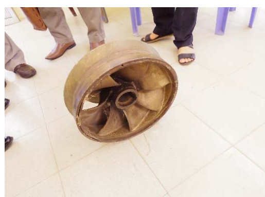
(Photo 4-19. Impeller removed for modifications)
