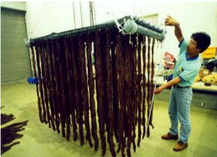
Photo 8-7-5 Artificial floating island utilizing string-like contact materials as dummy submerged plants
