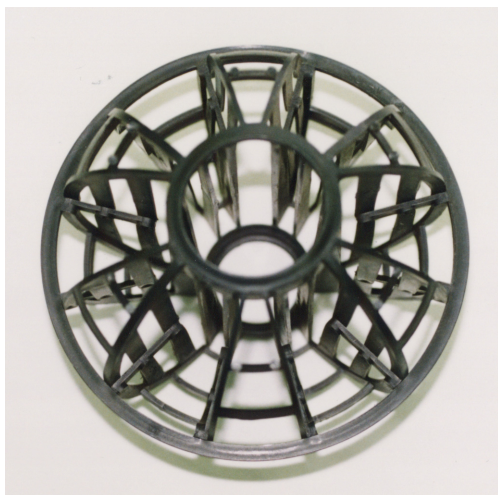
Photo 2-5-1 Media of fixed bed anaerobic reactor
