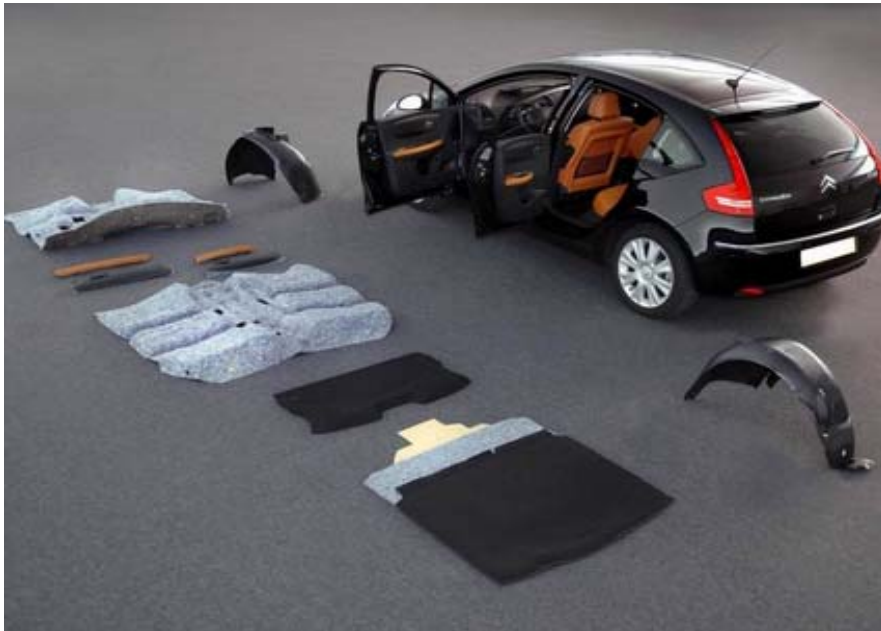
Examples of components used in the Citroën C4 containing green materials. (door insets, the rear parcel shelves, mudguards etc.)
