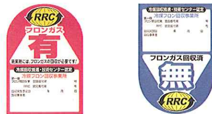
Fig. 7 Seal (Refrigerant charged, Refrigerant recovered)
