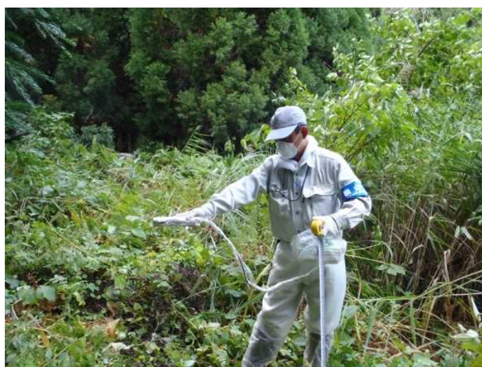
Figure 6. Measurement of ambient dose rates (example)
