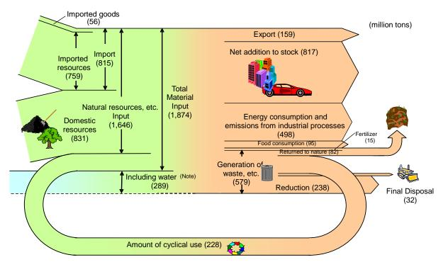
(Note) Including water: Input of water included in waste and the like (sludge, animal manure, human waste, waste acid, waste alkali) and sediment and the like associated with economic activities (sludge from mining, building and water works and tailing from mining).
