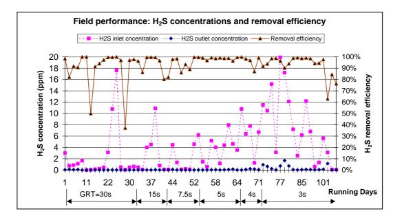
Figure 3 H<sub>2</sub>S removal efficiency with step-wise reduction in gas residence time (GRT)
