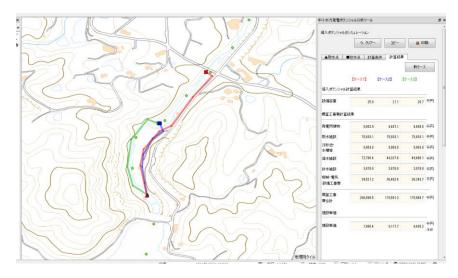
Fig. 2 Example of a newly added function (simultaneous display function for computation results)
