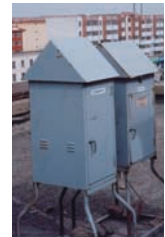
A high volume sampler for aerosol collection
