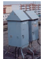
A high volume sampler for aerosol collection
